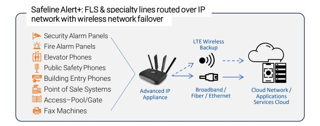
**Safeline Alert+** uses an enterprise-grade IP appliance that connects to your analog telephone and specialty lines, and analog traffic is converted to IP and sent over a VoIP network.
